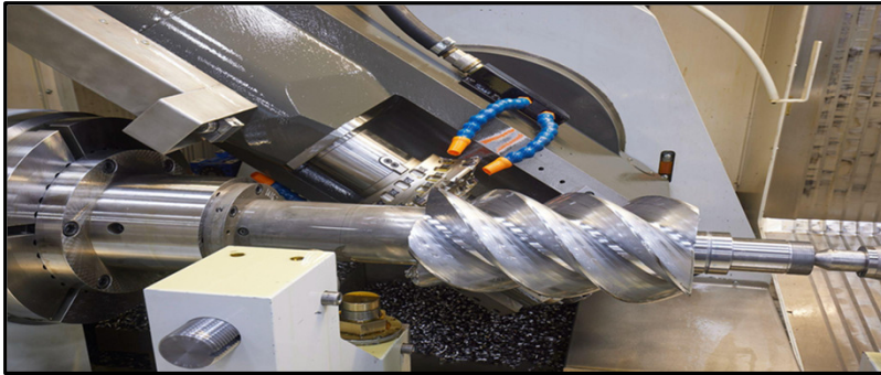
Screw Rotor Grinding using new Gen Machines
